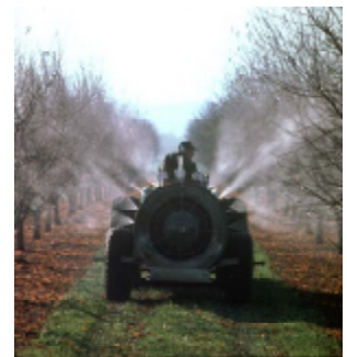
An air blast sprayer moves pesticide droplets high onto trees.
